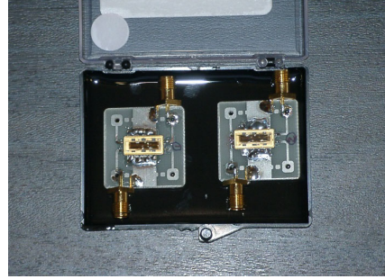
Fig.7 View of the Surface wave devices as mounted in the experimental bench
